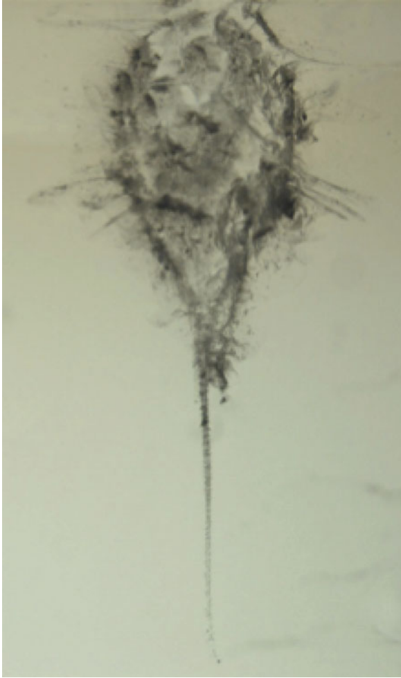
Fig. 5 Example of a track (C054-T3) in the Wild 2 aerogel collector. showing bulbous upper cavity with narrow tracks of terminal grains branching from it
